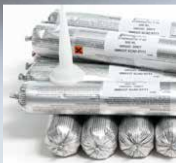
STARMASTIC P95 Polyurethane sealant medium modulus single component elastic, for floor joints or special gaskets. This sealant adheres directly to concrete, marble, stone, steel, aluminum, glass, resin, wood and plastic. It can be over-painted with elastomers and has excellent elasticity and resistance to chemicals and water.
